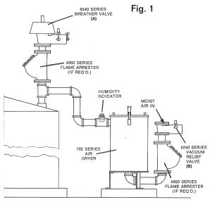
Above ground vertical tank shown. Above ground horizontal tanks and below ground tanks use the same equipment with modified piping arrangement.
